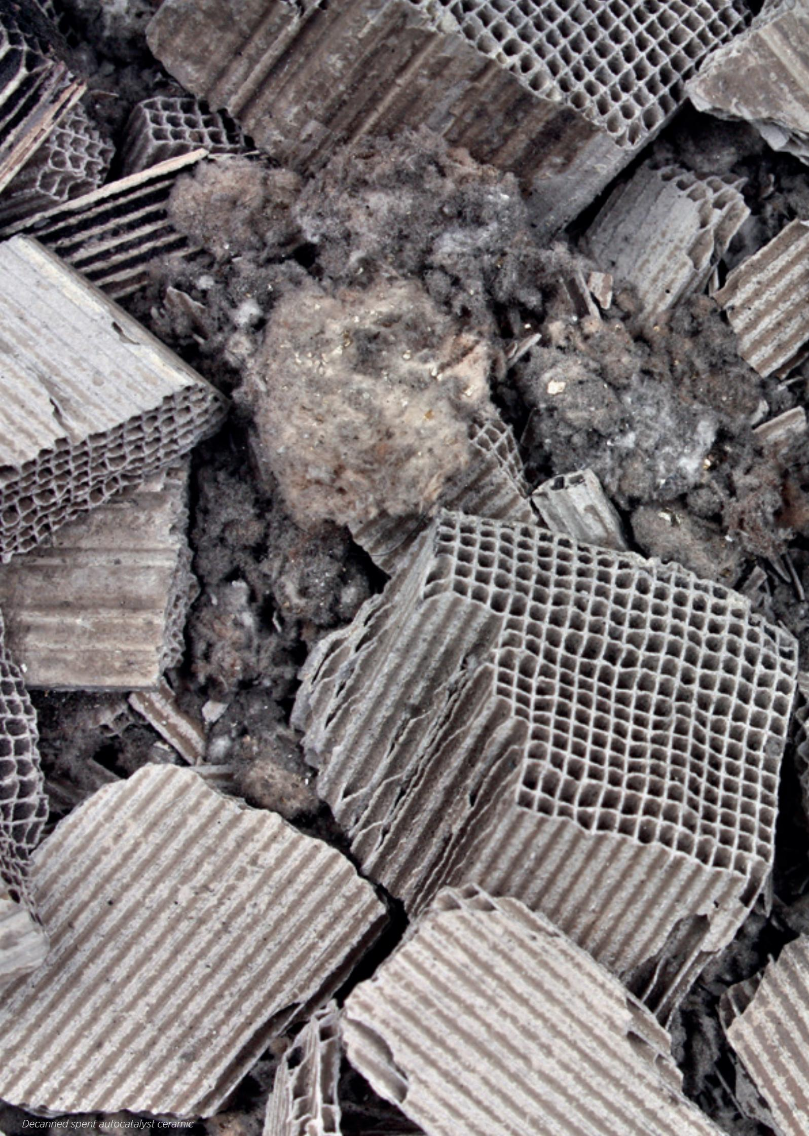
*Decanned spent autocatalyst ceramic*
